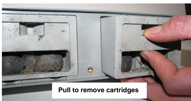
Carefully slide out both cartridges, remove the 4 balls.
